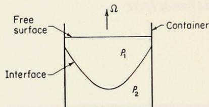
Figure 2. Observed interface displacement after the lower fluid has reached rigid-body motion and the upper fluid is still relatively motionless in the rest frame.
