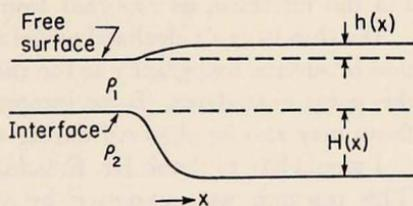
Figure 1. Inverse magnification of the surface topography over the layer of no motion.
