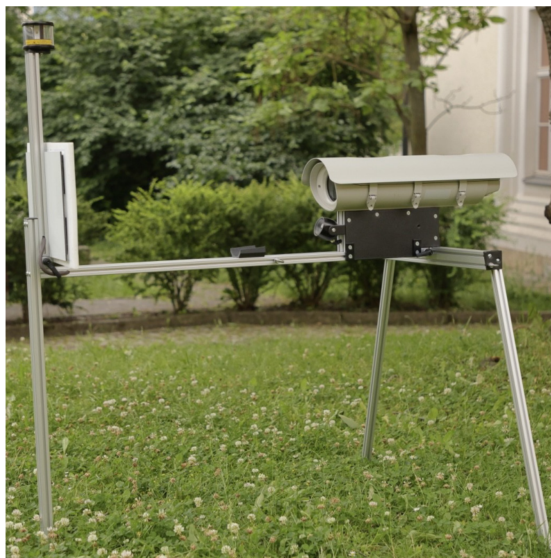
Figure. LEPMON'S current camera light trap (CLT) setup.
