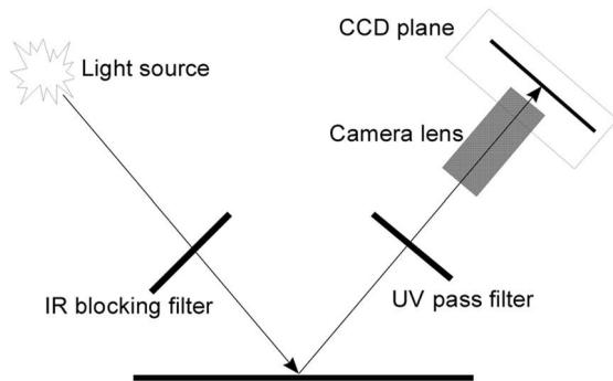
FIG. 3. Light path diagram for a typical UV imaging system.
