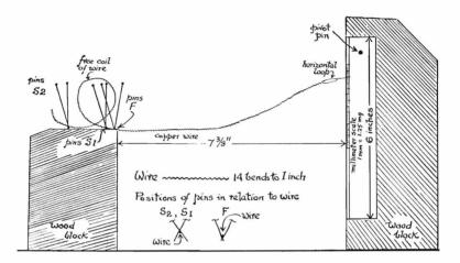
The scale is a millimeter rule, 6 inches long, held on the right-hand block by a pivot-pin near the top; this pin allows the scale to be moved to the right or left in an arc to adjust the millimeter marks to coincide with the end of the pointer when in the "rest" position.
