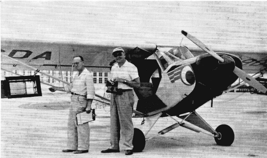
Fig. 1. Piper Cub plane equipped with insect traps placed beneath wings with control wires running from traps to cabin. A screen is partly pulled out of closed compartment for exposure as when in operation (Glick, 1955).
